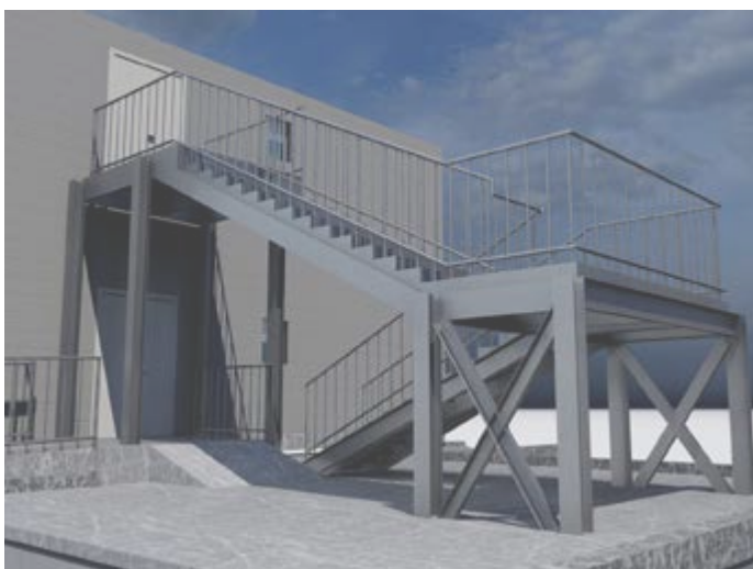
Example of 3D BIM model required: basic design representation of the external safety stair
